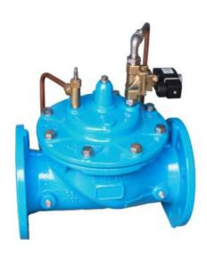
The Model 600 Solenoid Control Pilot Operated Valve is an on-off control valve that either opens or closes upon receiving an electrical signal to the solenoid pilot control. This valve consists of a main valve and two-way solenoid valve that alternately applies pressure to or relieves pressure from the diaphragm chamber of the main valve. It is furnished either normally open (de-energized solenoid to open) or normally closed (energized solenoid to open).
