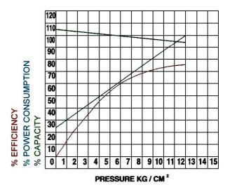
Looking at the curves one finds that pressure is the most important parameter in performance of a pump. It has different effect on different pump characteristics.
